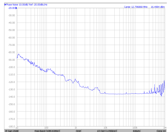
Figure 5. The phase noise of crystal oscillator with the vibration isolation system in the random vibration environment
